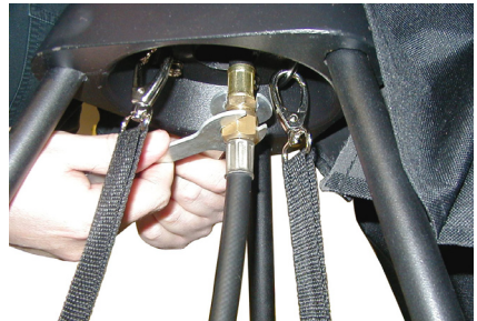
Figure 11 - Attaching Regulator Hose to Burner Fuel Line
